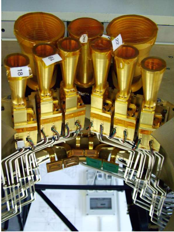
Fig. 12. Picture of nine of the eleven feed horns and associated OMTs, FEMs and waveguides before integration of the HFI front end. The six smaller feeds in the front are the 70 GHz channels, while in the back row are the two 30 GHz feeds and one of the 44 GHz feeds in the middle. Visible are part of the twisted Cu waveguide sections. The reference horns are visible (protected by a kapton layer): for the 70 GHz FEMs they are embodied in the FEMs, while for the 30 and 44 GHz they are flared waveguide sections.
